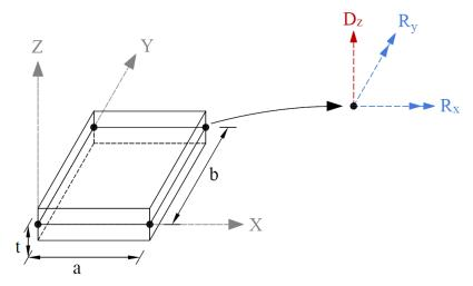
Figure 2.3 – Plate Finite Element
