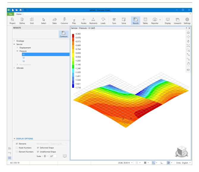
Soil pressure values in the contour view above differ along dissimilar soil boundaries. More information about Winkler's Foundation can be found in <u>Section 2.3.2.1</u>.
