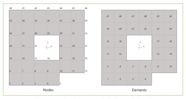
Figure 4.1 – Node and Element Numbering in Analytical Model
